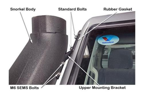
Install the ARMAX air ram assembly (Item 2) onto the snorkel body.
