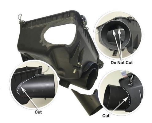
The following ribs on the air cleaner base must be removed or shortened as shown.
