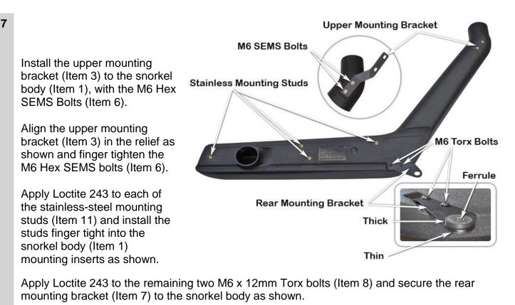
Install the rubber grommet (Item 9) into the lower mounting bracket (Item 7) with the thicker side of the grommet facing the panel side of the snorkel body.
