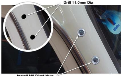
Drill a pilot hole at the rear mounting brackets (Item 7) lower marked hole position in the guard panel.
