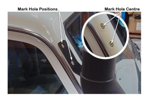
Mark the centre point of the two slots in the upper mounting bracket (Item 3) onto the vehicle A 'Pillar as shown.
