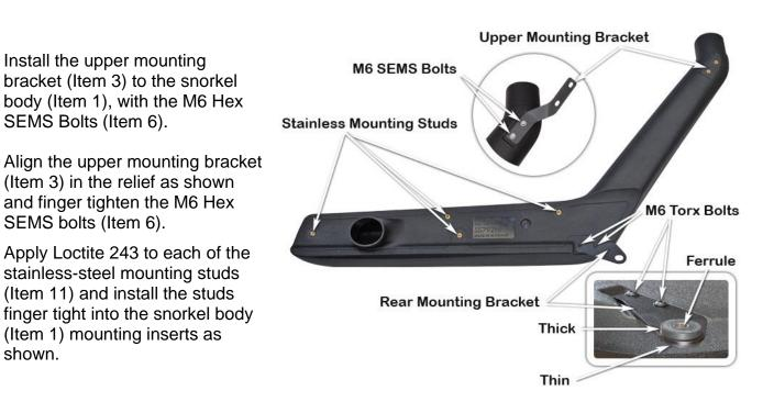
Apply Loctite 243 to the two M6 x 12mm Torx bolts (Item 8) and secure the rear mounting bracket (Item 7) to the snorkel body (Item 1) as shown.
