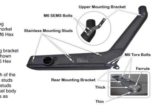
Apply Loctite 243 to the two M6 x 12mm Torx bolts (Item 8) and secure the rear mounting bracket (Item 7) to the snorkel body (Item 1) as shown.
