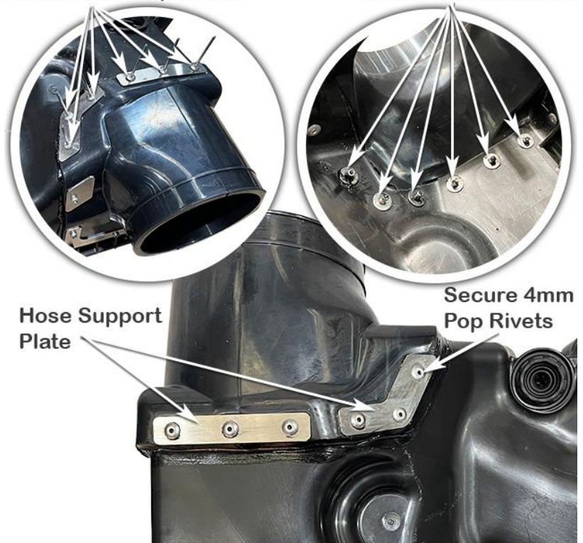
Install 4mm Pop Rivets
