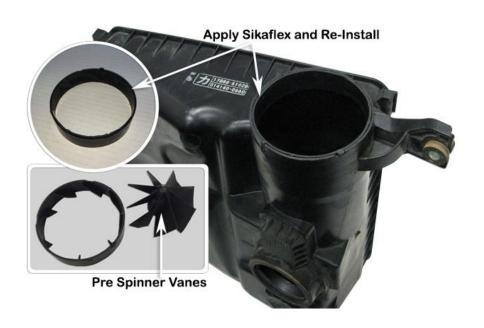
Using a scribe or paint pen, scribe or mark a line 18mm in from the end of the air cleaner inlet snout around the entire circumference as shown.
