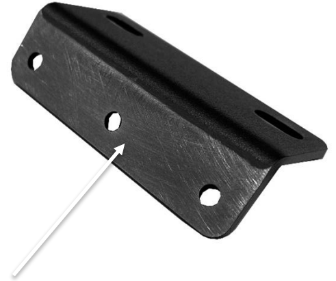
Powder Coating Removed
