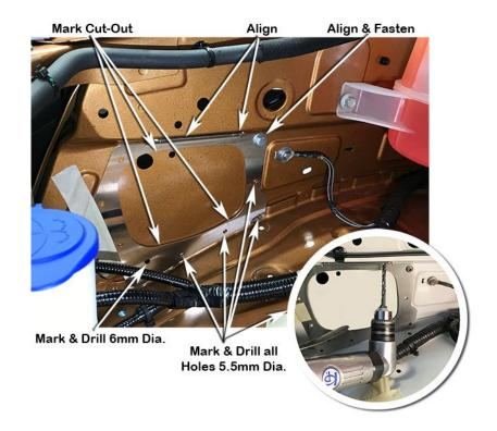
Using the body saw, cut the marked cut-out in the inner fender panel, cutting on the outside of the marked line.
