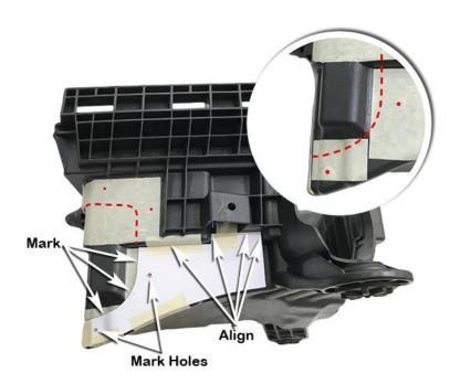
Neatly apply masking tape to the upper side surface of the air cleaner base, align the upper side template (item 29) to the air cleaner base as shown.
