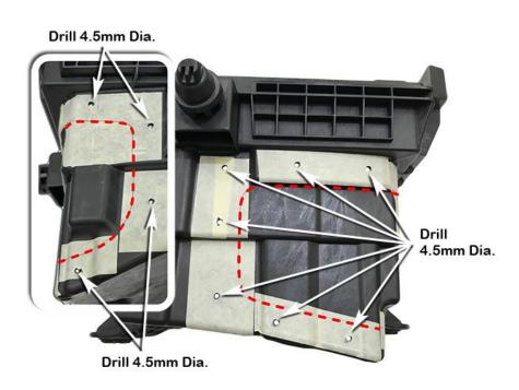
Using the body saw cut the new air inlet hole as marked from the templates in steps 18, 19, 20, & 21.
