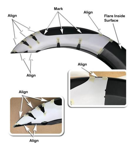
Using the body saw, cutout the marked section of the fender flare.
