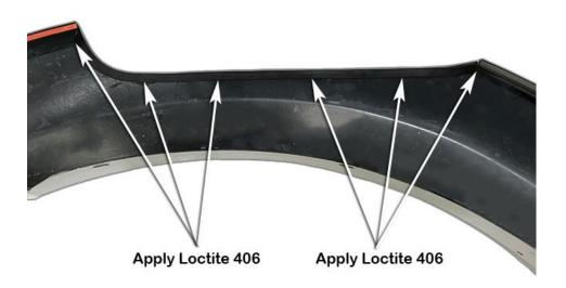
Install the flare to the vehicle as per the factory flare kit fitting instructions.
