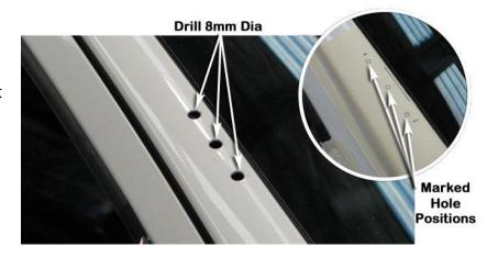
Install the plastic inserts (Item 6) into the 8mm diameter holes in the A-pillar.
