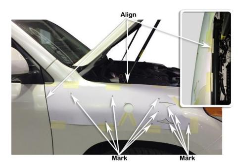
5 Drill a pilot hole for each of the marked positions.
