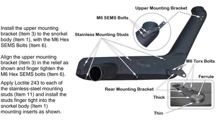
Apply Loctite 243 to the two M6 x 12mm Torx bolts (Item 7) and secure the rear mounting bracket (Item 5) to the snorkel body (Item 1) as shown.
