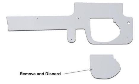
Align the guard panel template (Item 25) to the rear edge, upper edge and to the front factory hole of the guard panel as shown.
