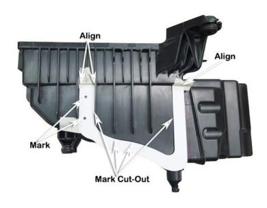
Using a body saw, remove the marked cut-out section of the air cleaner base.
