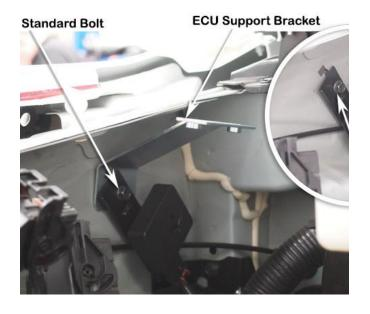
Install the ECU control module and bracket to the vehicle using the two standard 6mm hex bolts previously removed in step one.
