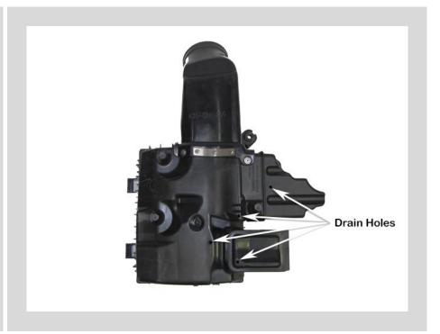
Correctly install the air cleaner base into the three rubber mounting grommets and secure with the standard mounting bolt.
