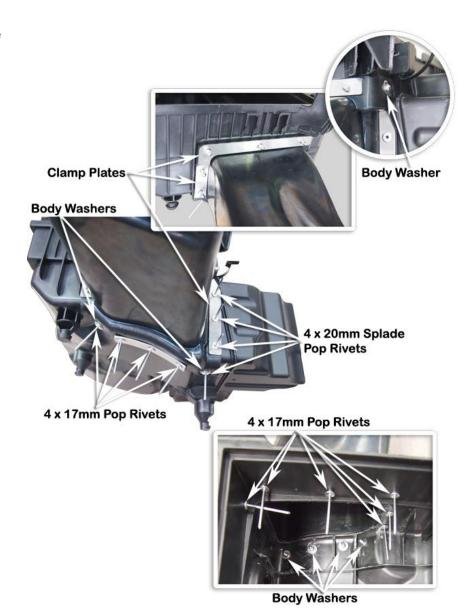
With all pop rivets, clamp plates and body washers in place, secure all pop rivets using a pop rivet gun. Clean-up any excess sealant to ensure a neat finish.
