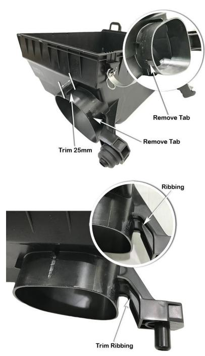
Using a grinder or file, remove the two retaining tabs from the air cleaner base inlet snout.
