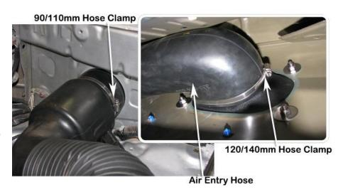
Install the black hose clamp (Item 13) loosely over the base of the air ram assembly (Item 2).
