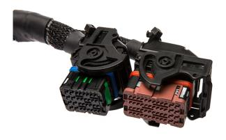
Now connect the 2 header connectors to the Bridge out connector as shown in the diagram. The inner connector has to be fitted first. The connectors only fit in one way and the lever arm must be all the way down. Push the header connector down into the bridge out connector until the lever arm covers the spigot. Then rotate the arm up towards the top of the connector until it locks. The connector will pull itself into location.
